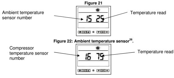
Figure 23: Compressor temperature sensor.
