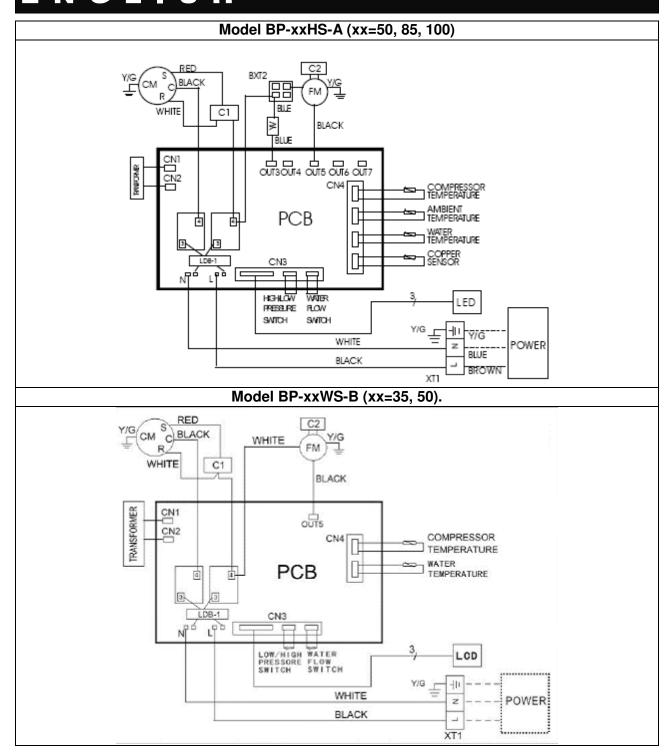
Figure 10: Wiring diagram.
