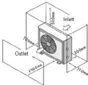
Figure 2: Clearance required for correct installation.
