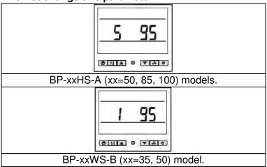
Figure 32: Parameter 5 settings (Parameter 1 for model BP-xxWS-B (xx=35, 50)), default settings.
