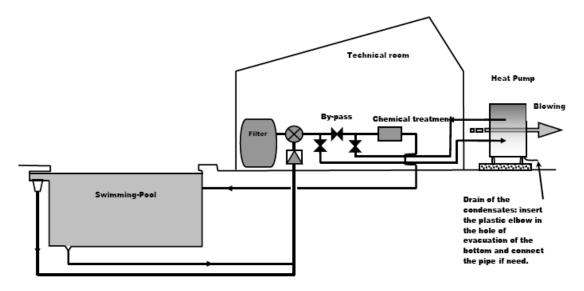
Figure 6: Typical hydraulic circuit part layout.
